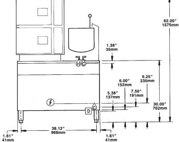
NOTE: When ordering optional reverse door openings: Control Panel, door openings, cooking compartments, clearances, and kettle are opposite that shown.
